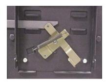
**Unlocking from the side**: Slide the tool in from the side. It will ride up over the lock and catch it. Pull the lock back to unlock.
